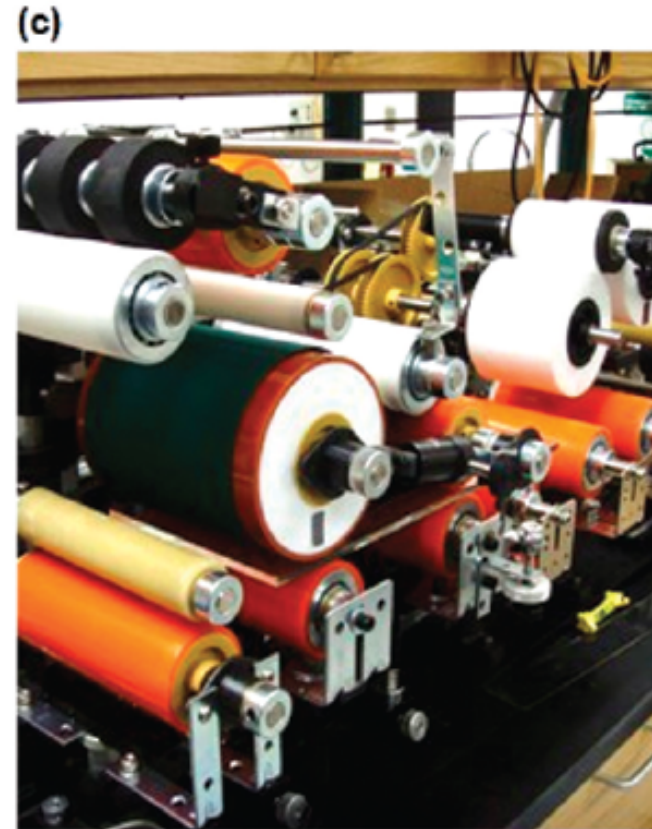
Figure 1. Schematics of (a) R2RNIL and (b) R2PNIL process. (c) Photograph of 6 in.-capable R2R/R2PNIL apparatus.
